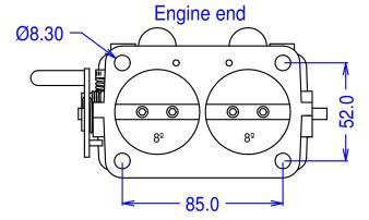
TheTC body is designed to fit the same flanges as twin downdraft DCNF carburettors from Weber. It is a compact body, well suited for use on 'V' engines with their tendency to long inlet tracts and shortage of space.
